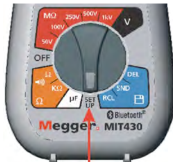
Selector switch set to Setup
